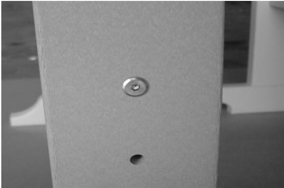
Place Leg Stretcher in between both Leg Assemblies. Align pre-drilled holes on Leg Stretcher to Leg Assemblies. Attach using (2) 3" Hex 1/4" Lags (Left Picture). Repeat process on all sides.
