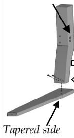
Insert left side Front Leg into threaded inserts in Left Arm as shown. Turn clock-wise until snug. Continue turning until legs are into aligned position. Secure with (2) 1-3/4" Phillips Head Screws.
