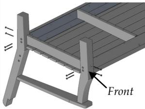
Lay seat upside down on a bench with side hanging over. Align Counter-bored holes in legs with pilot holes in aprons. Front of seat will be marked with an "F" on the bottom of the apron. Attach using (8) 80mm Hex Lags. Plug holes with 5/8" Bungs using rubber mallet.
