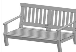
Attach Back to Mid Leg using (2) 1-3/4" Phillips Head Screws.
