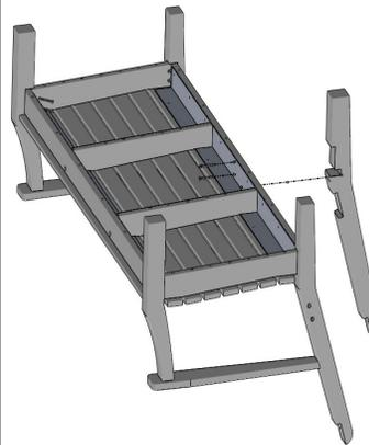
If you are assembling a Sofa (090), Align Mid Rear Leg with Rear Apron and Last Slat and Secure using (2) 2-1/2" Pan Head Screws thru holes in Rear Apron using a #3 Phillips Head Screwdriver.
