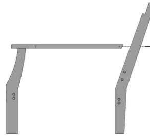
Align counter-bored hole in Rear Left Leg with Pilot hole in Left Arm. Attach using (1) 80mm Hex Lag. Plug holes with (1) 5/8" Bung using rubber mallet.
