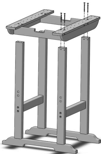
Align counter-bored holes in long apron assembly with Predrilled holes on Legs as shown. Secure using (8) 80mm Hex Lags.
