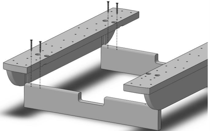
Align slots in long apron assembly with short apron. Secure using (8) 1-1/4" Phillips Head Screws through pilot holes in short aprons.
