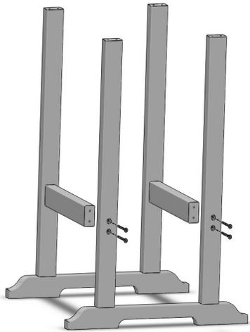
Attach Stretchers to Leg Assemblies using (8) 80mm Hex Lags (16 for Bar Height) as shown. Plug holes with 5/8" Bungs using Rubber Mallet.
