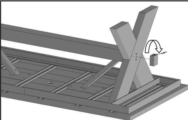
Insert End Caps into threaded insert in Leg Assembly. Turn clockwise until snug. Continue turning until in line with the Stretcher as shown. Secure end caps into legs with (4) 1-3/4" Phillips Head Screws.
