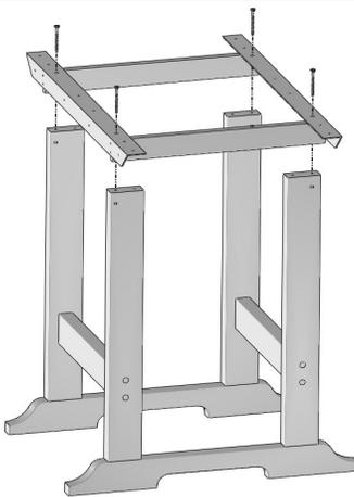
Align large holes in Aluminum Support Braces with Predrilled holes on outside corners of Legs as shown. Secure using (4) 80mm Hex Lags.
