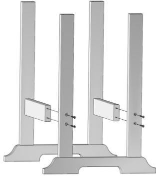
Attach Stretchers to Leg Assemblies using (8) 80mm Hex Lags (16 for Bar Height) as shown. Plug holes with 5/8" Bungs using Rubber Mallet.
