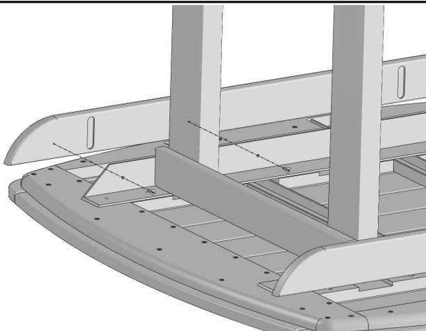
Align Long Aprons with Aluminum Support Brace. Ensure that pockets in Long Apron are aligned with Screws used to attach Short Aprons. Secure using (8) 3/4" Pan Head Screws thru Aluminum Support Brace.
