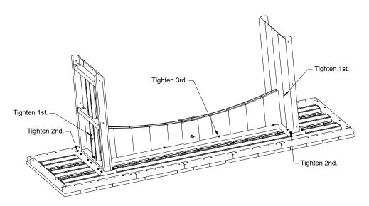
7. Attach Leg Cover to Leg with 6- 2 1/2" wafer bolts per leg.
