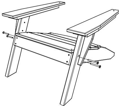
2. Assemble 2 - 2-1/2" Screws per side of Seat Support in pre Drilled Holes.
