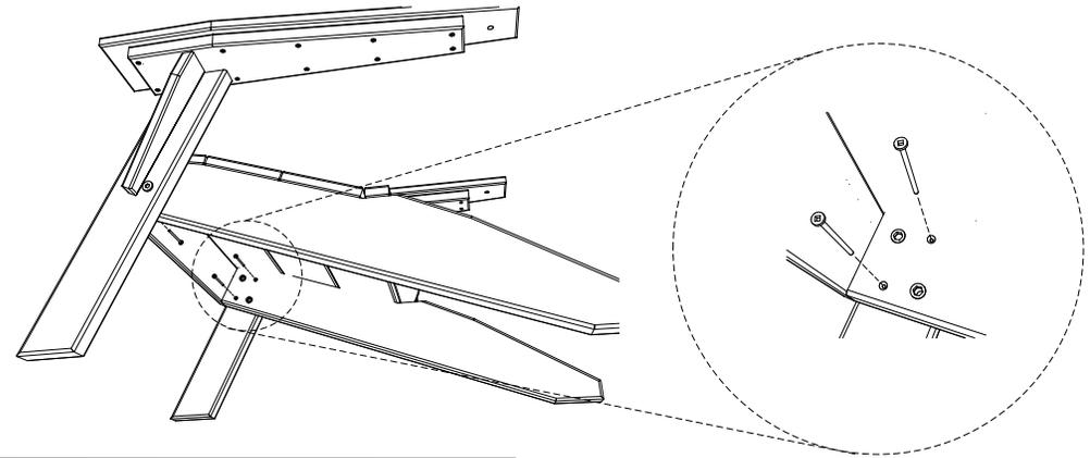
3. Attach (B) Back Assembly using 1 - 1-3/4" Stainless Wafer Bolt and 2 - 2" Stainless Steel Screws per side, Be Sure to match all numbers and or letters.
