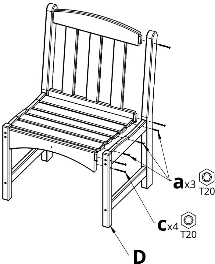
**3.** Attach Part F using the hardware shown
