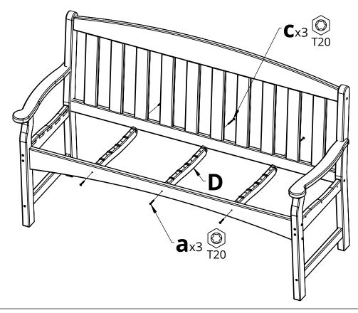
**2.** Connect Parts D to the prevoius assembly as shown
