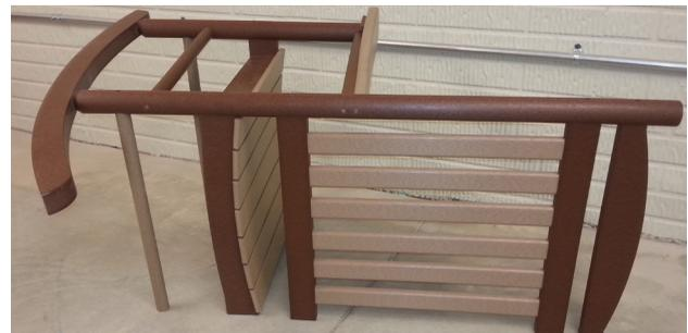
(B) Place the long footrest in mortise in the front leg and the short footrest in mortise in back leg and fasten each footrest to leg with (1) 3" screw.
