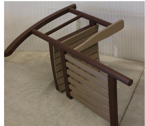
(B) Place the rocker back into the mortises located on the back leg of rocker and fasten in place with (2) 3" screws.
