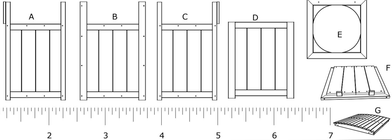
1. Attach (B) Front Panel to (A) & (C) Side Panels using 4 - 2" Screws in predrilled Holes. See Notes
