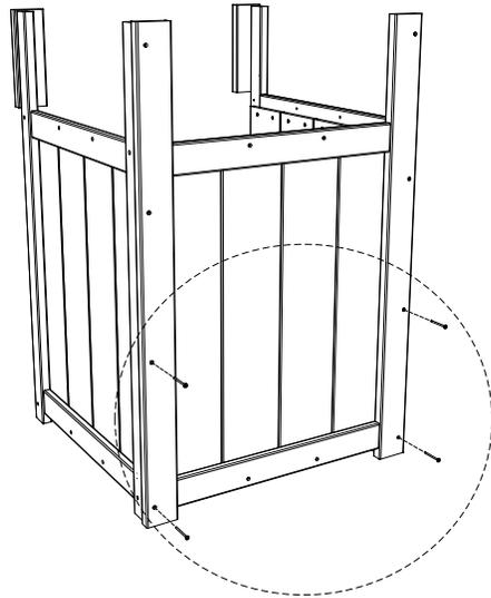
Note: Only attach bottom 2 Screws on each side as shown.
