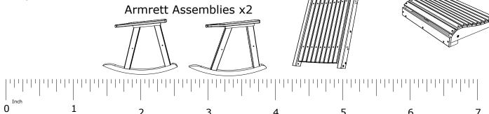
1. Attach Back Assembly to Seat Assembly Using 2 - 2 1/2" Wafer Bolts per side, tighten Wafer Bolts with included Hex Key. Be sure to match all numbers.
