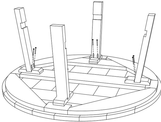
2. Attach (B) Shelf to (C) Legs using 2 - 2" Screws Per Leg.
