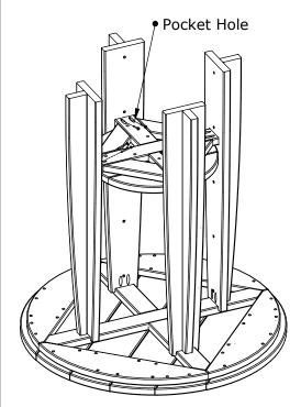
3. Attach Braces using 1-1/2" Screws in predrilled holes. Keep Braces centered with legs & Crosspiece.
