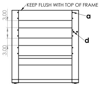
**6.** Insert sling spacer **D** into the seat frame as shown at left. Be sure it is pushed against the back of the seat. Install (6) hardware C to hold it in place. Insert the seat sling (C) into the seat frame. It should drop into the frame with minor pressure applied to the frame sides.
