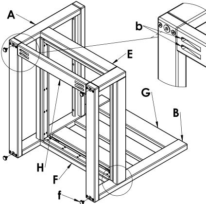
(2) 1-3/4" screws (**b**) are used on each end of **E**, **F** & **H**.
