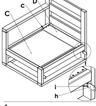
**Optional:** If you wish to physically connect multiple pieces of furniture together, use the included plates and 1-1/4" screws (**h** & **i**) as shown at left. Connect plates to the inside faces of the front and back legs allowing approximately 1-1/2" of the plate to protrude from the side of the chair. Then move the next furniture piece into place and fasten the plates to it.
