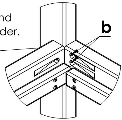
**3.** Using the 6" torx bit (hardware **f**), screw the (12) 1-3/4" screws (**b**) into the bottom spreader (**F**) and sling rails (**D**). When tight, the ends of the spreader and rails should be flush to the two side frame assemblies.
