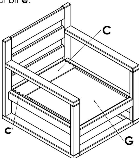
**6.** Insert sling spacer **C** into the seat frame as shown at left. Be sure it is pushed against the back of the seat. Install (6) hardware **C** to hold it in place.
