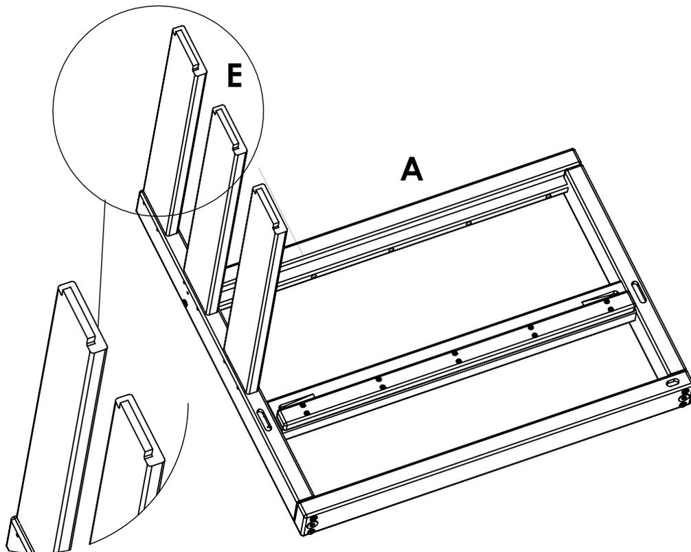
**2.** If you did not start with the slats on the floor, carefully rotate the chair to its back. Align the top back slot of assembly **B** with the top back slat. Align the remaining slats and use a mallet to start the slat tenons into the frame, leaving them slightly out.
