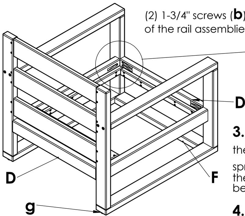
(2) 1-3/4" screws (**b**) on each end of the rail assemblies and spreader.
