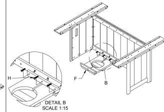
5. Attach (B) Front Panel with the Door to (A) & (D) End panels using 8-(G) 2" Screws in predrilled holes.
