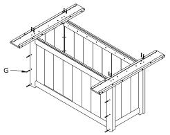
6. Attach Front Side of (F) Floor to (B) Front Side Panel using 3-(H) 5/16"X 1 1/2" Wafer Bolts.
