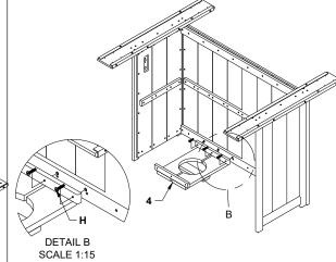
5. Attach (B) Front Panel with the Door to (A) & (D) End panels using 12-(G) 2" Screws in predrilled holes.
