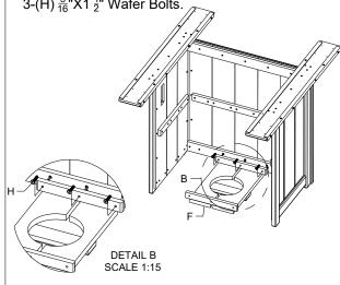
5. Attach (B) Front Panel with the Door to (A) & (D) End panels using 10-(G) 2" Screws in predrilled holes.
