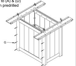
6. Attach Front Side of (F) Floor to (B) Front Side Panel using 3-(H) 5/16"X 1 1/2" Wafer Bolts.
