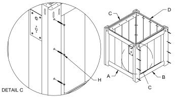
6. Attach Front Side of (F) Floor to (B) Front Side Panel using 3 (I) 5/16"X 1 1/2" Wafer Bolts.
