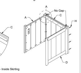
4.Attach 1 side of the (F) Floor to backside using 3 (I)  $\frac{5}{16}$ "X1  $\frac{1}{2}$ " Wafer Bolts.
