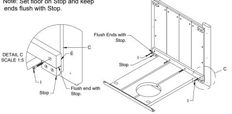
4. Position Aluminum Angle (E) into Notch of (A) Left End. Note: Push (A) Left End against Notch and Stops before attaching, using 2 (H)  $\frac{3}{4}$ " Screws. Attach (A) End Panel to (C) Back Panel using 3 (K) 2" screws in predrilled holes.
