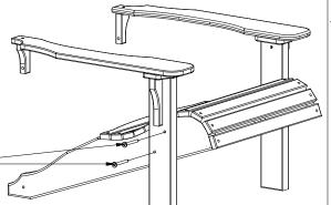
2. Attach Back Legs using 1 - 2-1/2" Wafer Bolt 1 - 2" Wafer Bolt & 1 - 2" Screw per side Tighten Wafer Bolts with included Hex Key, be sure to match all numbers.
