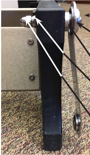
\frac{5}{16} X2- \frac{1}{2} " Allen Head Bolt Glider Bracket \frac{5}{16} " Aluminum Spacer \frac{5}{16} " Lock Nut \frac{5}{16} " Acorn Nut
