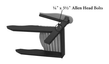
**STEP #1 -** Fasten the seat and the Arm Assemblies using two ¼" x 3½" Allen Head bolts.
