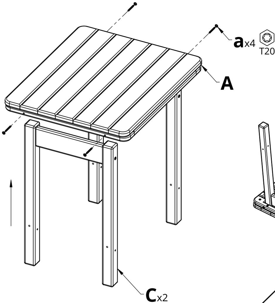
**1.** Attach Parts C to Part A using Hardware a
