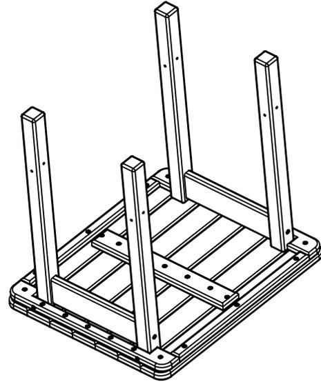
**3.** Attach Part D to the previous assemblies using Hardware c.
