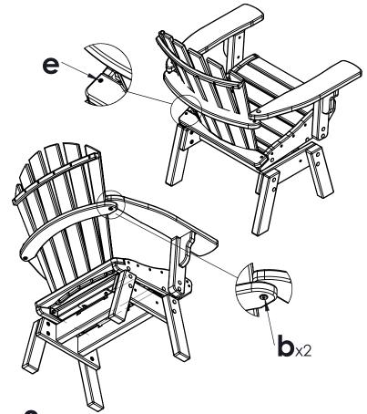
**9.** Attach Back Assembly I to the seat base using hardware **e**, 1 per side. Attach the Back Assembly center support to each arm using hardware **b**.
