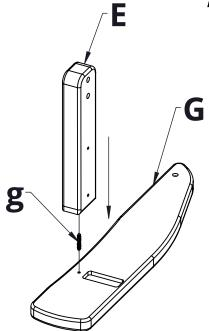
**4.** Attach Part **E** to Part **G** using Hardware **f**
