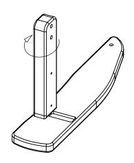
**5.** Rotate Part **E** clockwise until tight in the orientation shown
