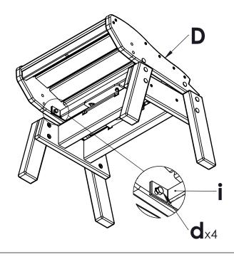
**3.** Attach Seat Assembly **D** to the swivel assembly **i** using Hardware **d**.
