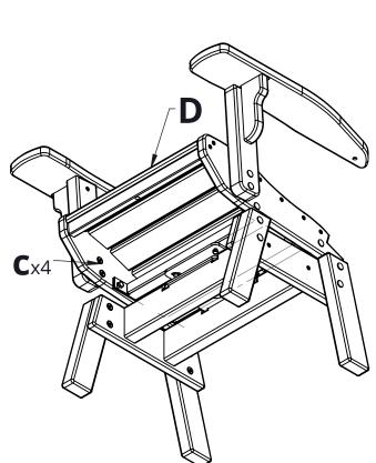
**8.** Attach the two arm assemblies to the seat base using hardware **c**.
