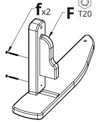
**6.** Place Part **F** into the pre cut slot and attach with Hardware **f**
