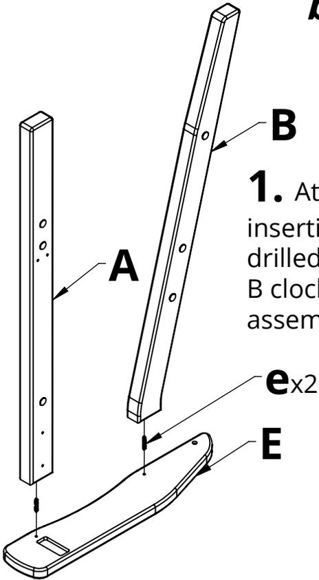
**1.** Attach Parts A & B to Part E by inserting Hardware e into the pre-drilled holes and rotating Parts A & B clockwise, stopping when the assembly is tight
