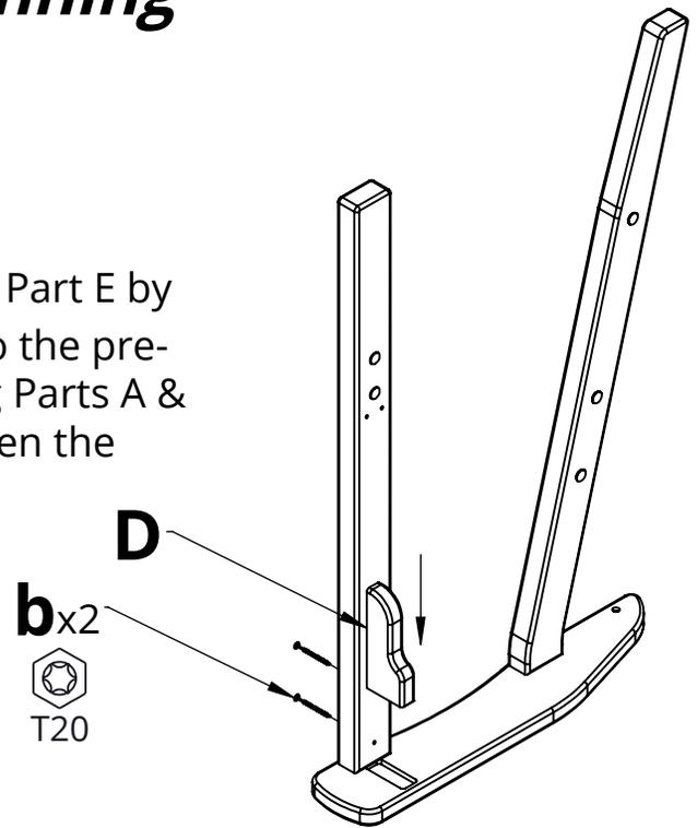
**2.** Attach Part D to the previous assemblies using Hardware b
