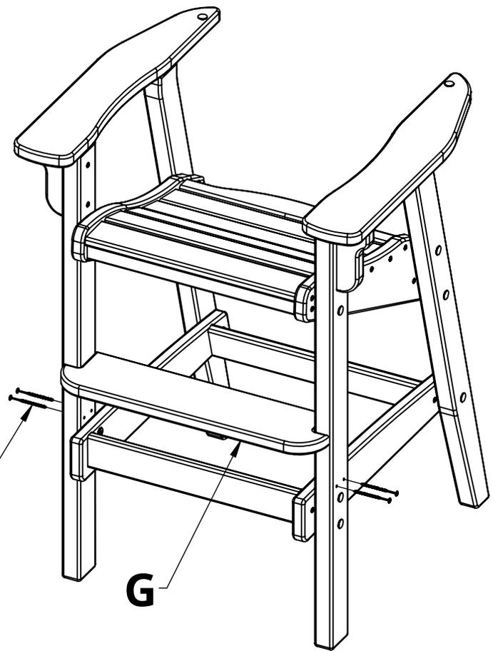
**6.** Slide part J into place and connect it as shown
