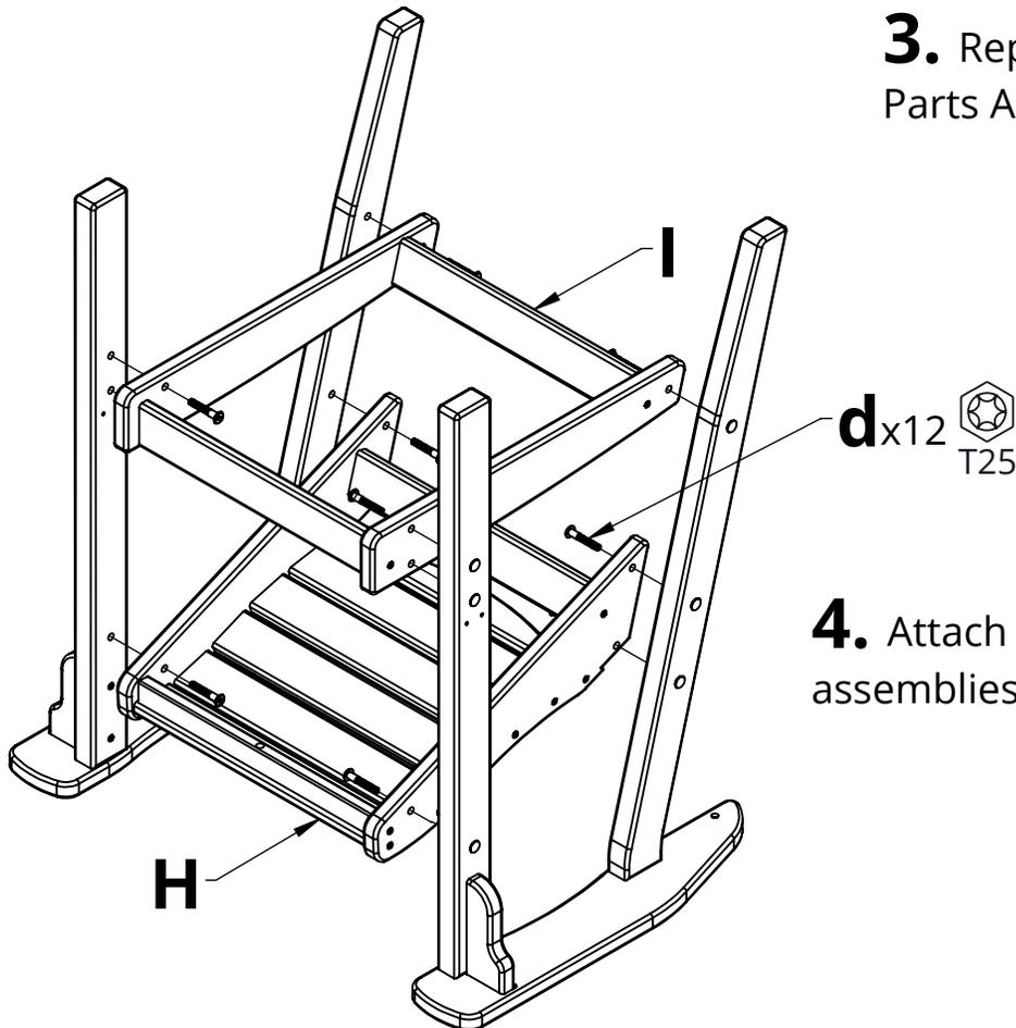
**4.** Attach Parts H & I to the previous assemblies using Hardware d
