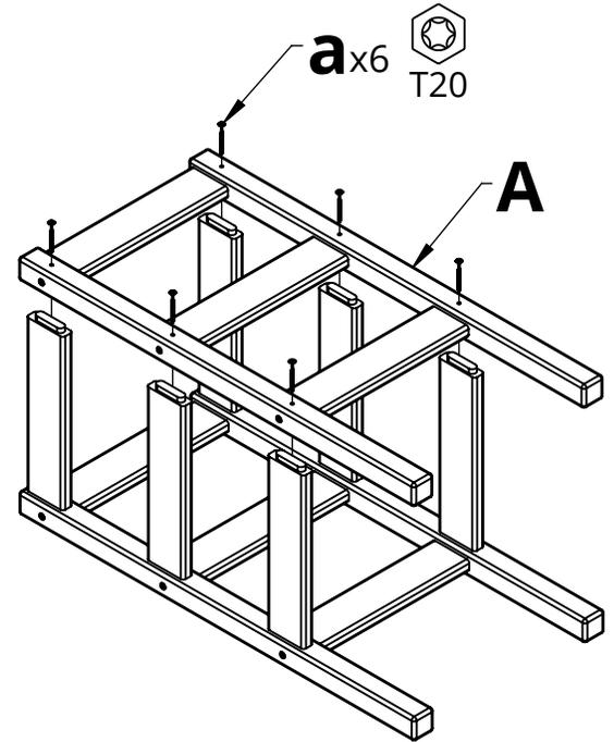
**2.** Place part A on top and connect with the hardware shown
