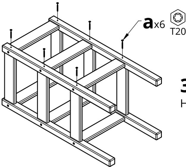
**3.** Turn the assembly over and insert Hardware a
