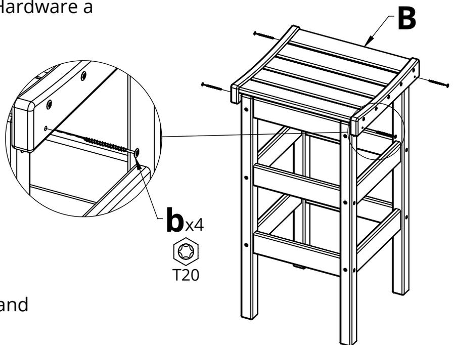
**4.** Stand the assembly upright and connect Part B with Hardware b
