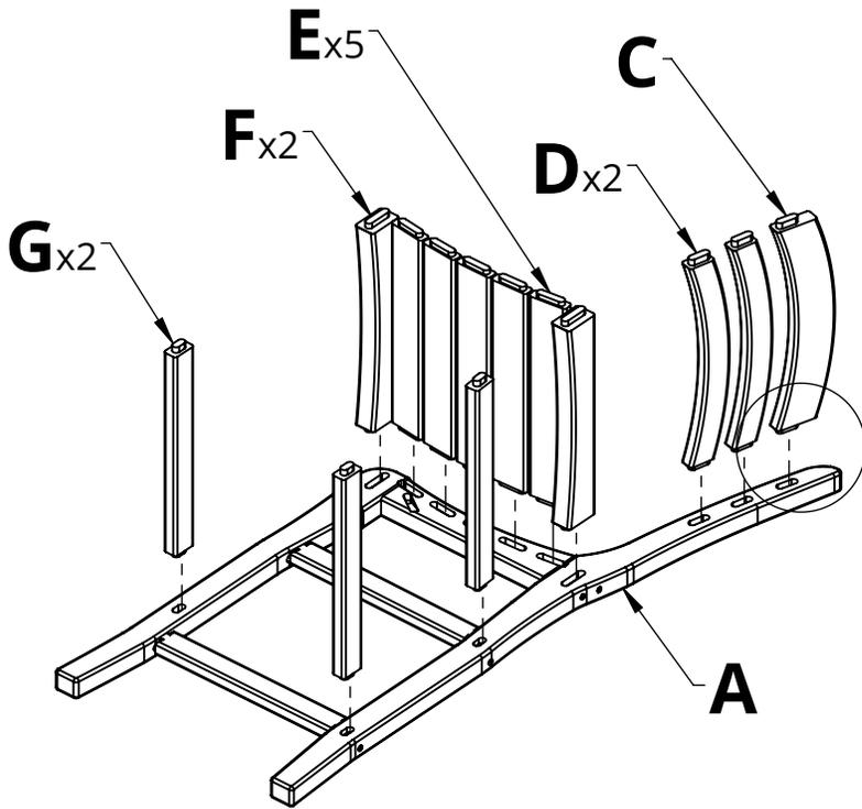
**1.** Place Part A on its side and place all Parts in as shown
