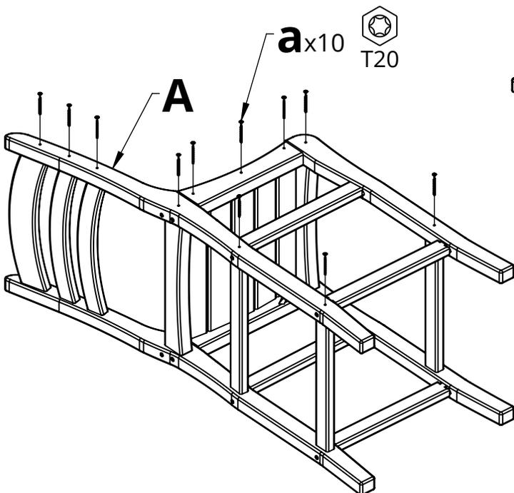
**3.** Turn the assembly over so Part A is up & connect it using Hardware a
