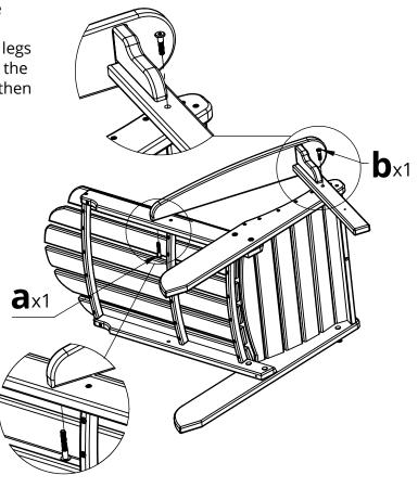
**8.** Assemble Part E into the chair. Insert the tenon into the slot in one leg. Then with slight pressure on the opposing leg, push the opposite side of Part E into its corresponding slot. Screw in place using 2 of hardware e.
