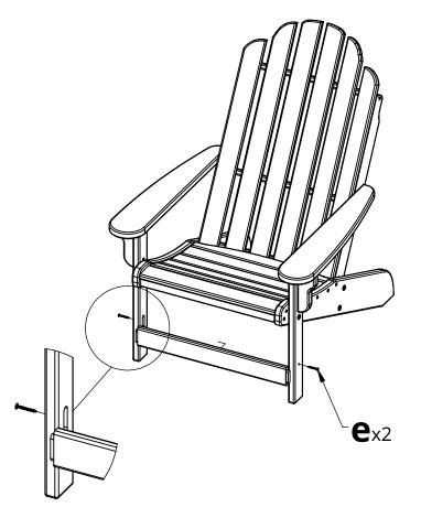
**7.** Turn the back/seat assembly on it's side. Lay one arm/leg assembly from steps 1-5 on the back/seat assembly and bolt together using 1 each of hardware a & b as shown. Flip the chair to the opposite side and repeat.
