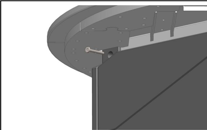
Drop Top onto Base and Secure using (4) 50mm Lags. Plug holes with 5/8" taps®.
