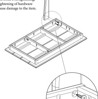
Use 2 of the 1/4" x 1 1/2" Wafer Head Lags as shown utilizing the provided 5/32"
