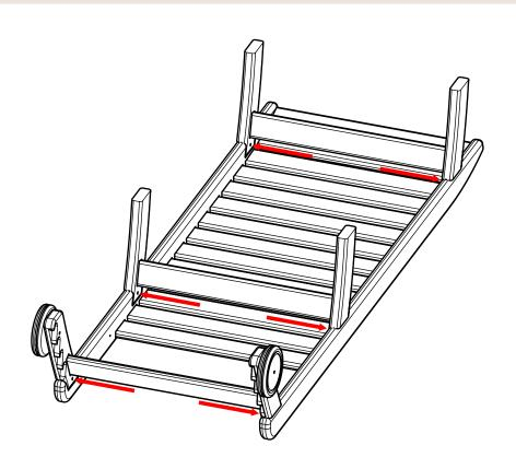
Slide the back into place. Make sure the seat is upside down on a nonmarking surface, then slide the back in until the slats are spaced evenly.
