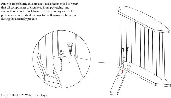
Use 2 of the 1 1/2" Wafer Head Lags as shown utilizing the provided 5/32" Allen Wrench.
