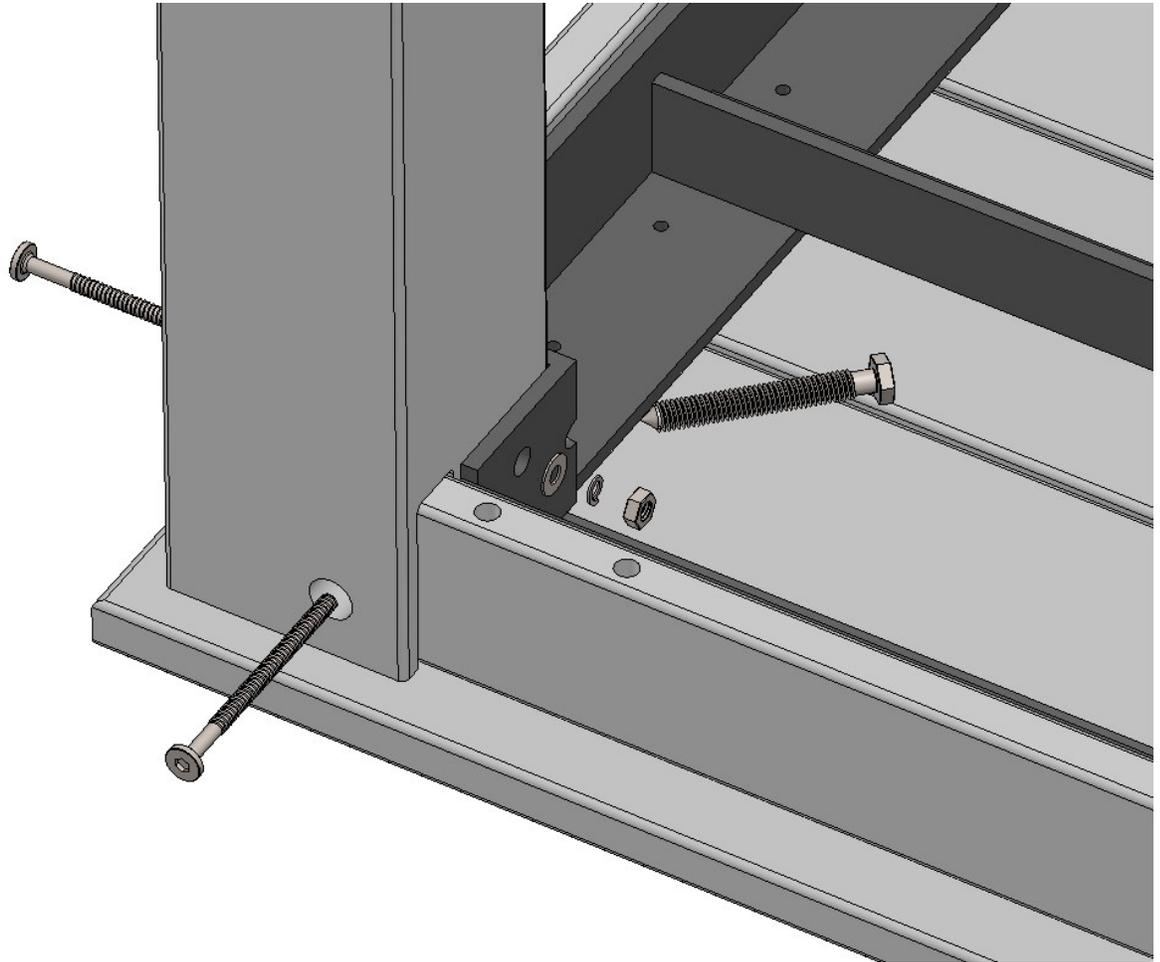
On a clean flat surface connect legs to Top using (2) 90mm Bolts, Washers, split washers, and nut (AS SHOWN). Finger tighten. Attach 3/8" LAG to inside of leg. Repeat with remaining legs. Do not over tighten. Plug holes with supplied 5/8" TAPS.
