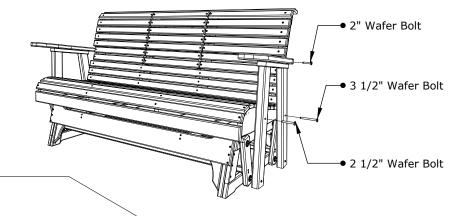
7. Attach Lintels to Armrest Assemblies using 4 - 2" Screws per side, be sure to match all letters.
