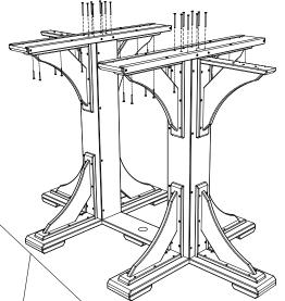
8. Align Stabilizer Block with Hole in Top, Attach Stabilizer Block using 4 - 2-1/2" Screws.
