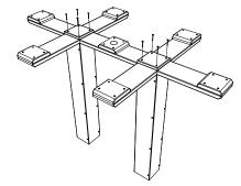
4. Attach 6 Braces to Pedestal Column using 6 - 1 1/2" Screws per Brace in predrilled holes, Be sure to center brace on Pedestal Column & keep top side flush.
