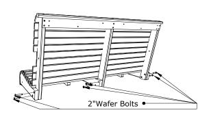
2. Attach Armrest Assemblies to each side using 1 - 3 1/2" Wafer Bolt 1 - 3" Wafer Bolt 2 - Washers & 2 Nuts per side. Be sure to match all letters Tighten Wafer Bolts with included Hex Key. :Insert Bolts from inside out:
