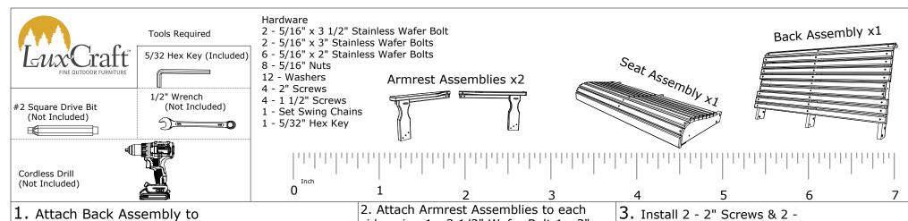
1. Attach Back Assembly to Seat Assembly using 6 - 2" Wafer Bolts, Be sure to match all letters, Tighten Wafer Bolts with included Hex Key.
