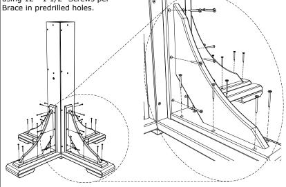
4. Attach Brace's to top of Pedestal Column using 6 - 1 1/2" Screws per Brace, Be sure to center Brace on Column & keep top side flush with Pedestal Column.
