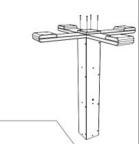
3. Attach Brace's to Pedestal Column using 12 - 1 1/2" Screws per
