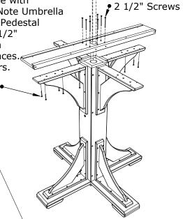
6. Align Top Short Crosspieces with Braces keeping back end flush with Top Long Crosspiece Attach using 12 - 1 1/2" Screws. Make sure that Aluminum is on top side.
