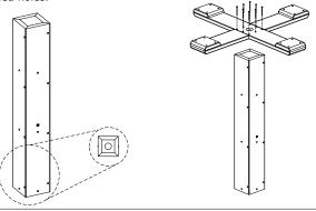
2. Align Pedestal Block in center of Pedestal Feet. Attach Pedestal Block using 4 - 1 1/2" Screws.
