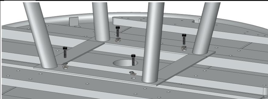
On a clean flat surface connect legs to top using (4) M6 Shoulder Screws, (4) M6 Lock Washers & (4) 1/4-20 Flat Washers (AS SHOWN). Do Not Over Tighten.
