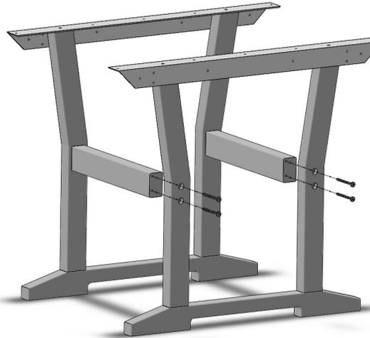
Attach Stretchers to legs through counter-bored holes in legs into pilot holes in stretchers using 80mm hex lags.
