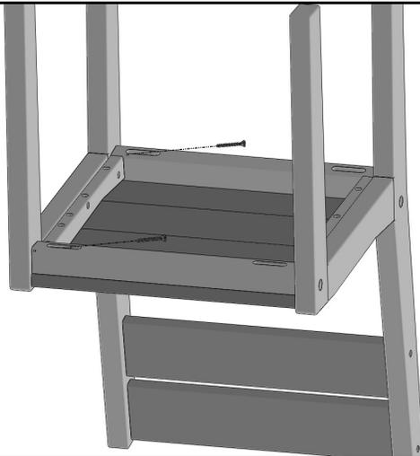
At this time make sure lags from step 2 are tight. Rotate rear apron to align with angle on seat support, and make sure front apron is parallel with front leg. Secure aprons with 1-3/4" Phillips head screws through the pockets on underside of aprons into legs.
