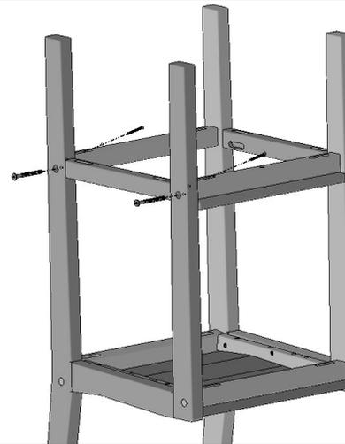
Attach Foot Rest and Rear Stretcher as shown, with pockets of Stretchers facing down, using (4) 80mm Hex Lags through counter-bored holes in Legs. Align straight, then secure using (4) 1-3/4" screws through pockets on underside of Foot Rest and Rear Stretcher.
