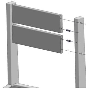
Tap 5/16" dowels into large holes in back slats. Align with large holes in rear legs. Secure with 1-3/4" Phillips head screws through 3/8" counter-bore in Rear Legs into pilot holes in back slats.
