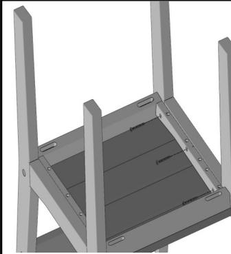
Align seat assembly with frame. Secure using 1-3/4" Phillips head screws through countersink holes on inside of seat assembly into pilot holes in side assemblies.
