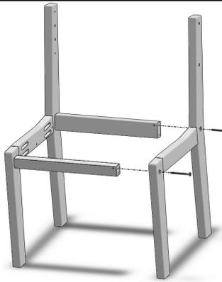
Attach front and rear aprons to Side Assemblies as shown, with the pockets of the aprons facing down using (4) 80mm Hex Lags through counter-bored holes in Legs.
