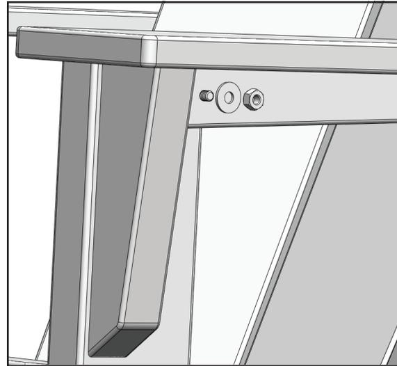
Place Arm on top of Front Leg. Align pre-drilled holes. Install a 60mm connector bolt, starting from the Front Leg through the Underarm. Finger tighten flat washer and Lock Nut. Do not fully tighten at this time. Repeat process for opposite Arm.
