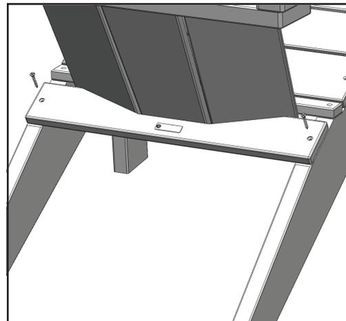
Place Back Assembly on top of mounting surface of Rear Legs (Part of Seat Assembly). Push Back Assembly forward until it meets the last Seat Slat of the Seat Assembly. Hold Back Assembly in place and install (2) 1-3/4" Phillips Head Screws into pre-drilled holes on each side of the Lower Yoke (No pre-drilled holes on Rear Legs).
