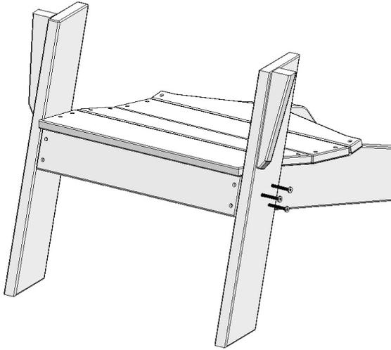
Attach using (3) 75mm connector bolts through the pre-drilled holes. Finger tighten flat washer, lock washer, and attach nut on each bolt. Do not fully tighten at this time. Repeat process for opposite Leg.
