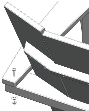
Place Upper Yoke of the Back Assembly underneath arms, aligning pre-drilled holes. Install (1) 60mm connector bolt through pre-drilled hole of the Arm and through Upper Yoke. Finger tighten flat washer and Lock Nut. Do not fully tighten at this time. Repeat process for opposite Arm.
