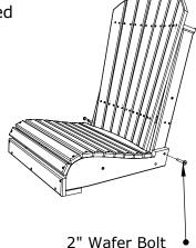
3. Slide Seat & Back Assembly between Armrests & attach to Armrests using
