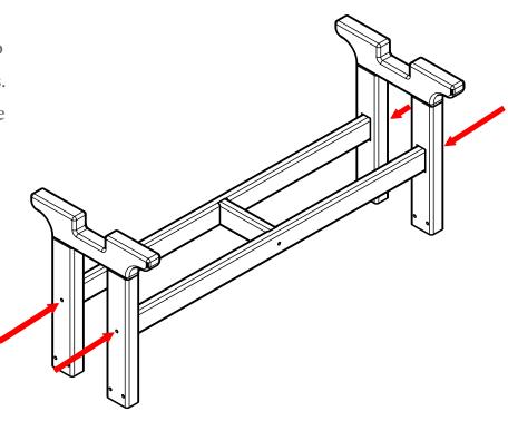
Use eight 2" wafer head lags to attach the legs to the bench top.
