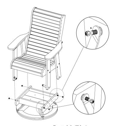
Ten attach the Glider Arms to all 4 carriage bolts on the base and finally securing them with 5/16" Lock nuts.
